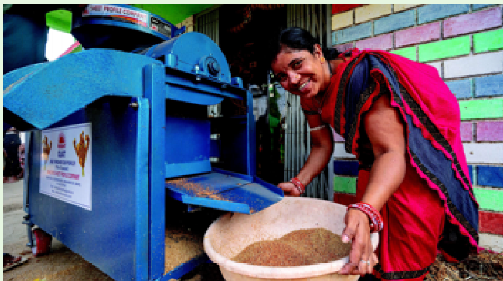
A member of Maa Bastarani Self-Help Group operating Thresher-cum-Pearler to separate Ragi grains at Belagaon village in Komna Block of Nuapada District.
