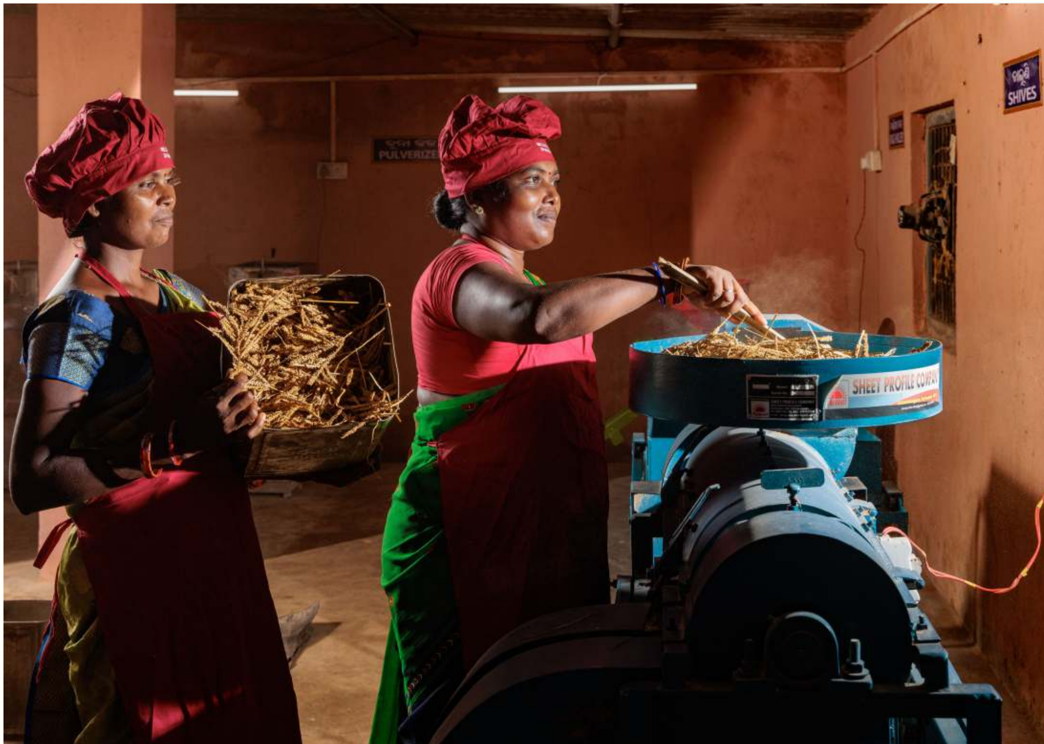
WSHG members threshing the finger millet ( Ragi ) with help of Thresher cum Pearler developed by Odisha University of Agriculture & Technology.
