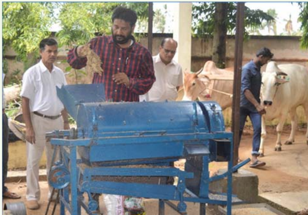
Demonstration of Sorghum thresher cum cleaner operated by bullock power in rotary mode in CAET premises
